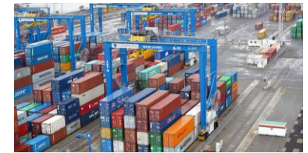
Fully-electric ARTG (cable reel)
